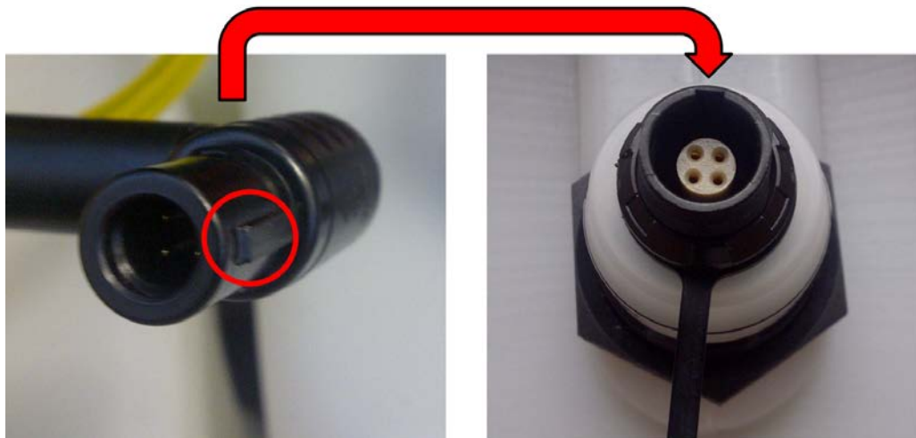
Figure 5-37: Sensor connector alignment
